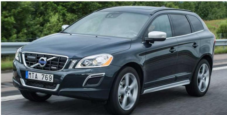
A highlight for a brand specifically known for safety technology, the XC60 was the first vehicle in Volvo's lineup equipped with City Safety, a driver support system aimed at preventing or mitigating collisions occurring at speeds of 19 mph or less by actually automatically braking the XC60 to help avoid a rear-end collision or lessen its impact. Underhood, the XC90 offers a choice of an entry-level 230-horsepower 3.2-liter PZEV naturally
