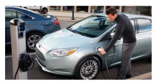
Powered by 23kWh Lithium-ion battery pack, the **2014 Ford Focus Battery Electric** hatchback features a liquid cooled and heated battery pack intended to deliver consistent driving ranges over a wider spectrum of temperatures — and a top speed of 84mpg. Thanks to its giant potential 19.1 percent discount off the \$35,995 MSRP, the electric
